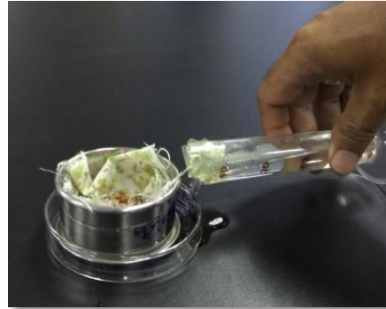
(iv) Adding water to touch bottom of the sieve and muslin cloth
